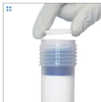
Add a top frit on the added media and align the frit horizontally.
